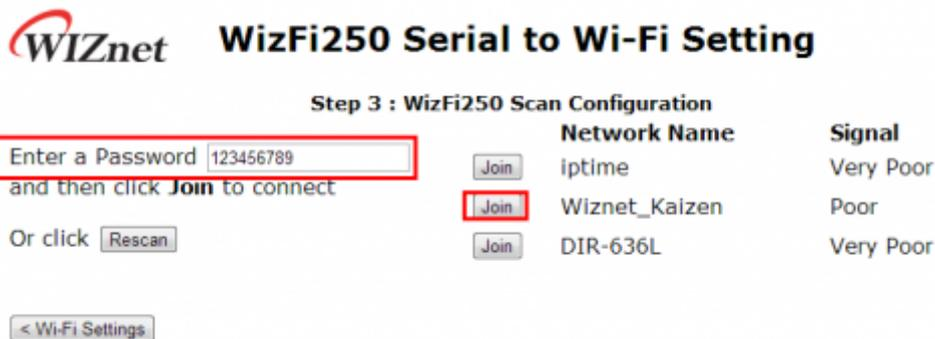
If you can see “Device Started. Web server and access point stopped. See UART for further information.” message in the web browser and “Successfully joined” message in the serial terminal, WizFi250 is associated to AP successfully.
