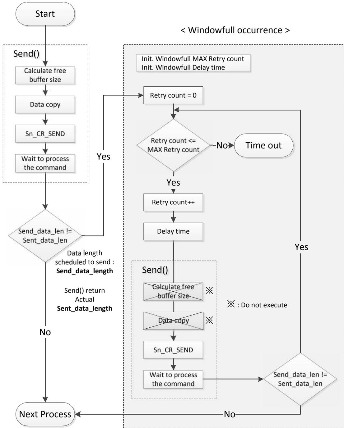
Fig. 2.2 SEND() : Windowfull handling process
