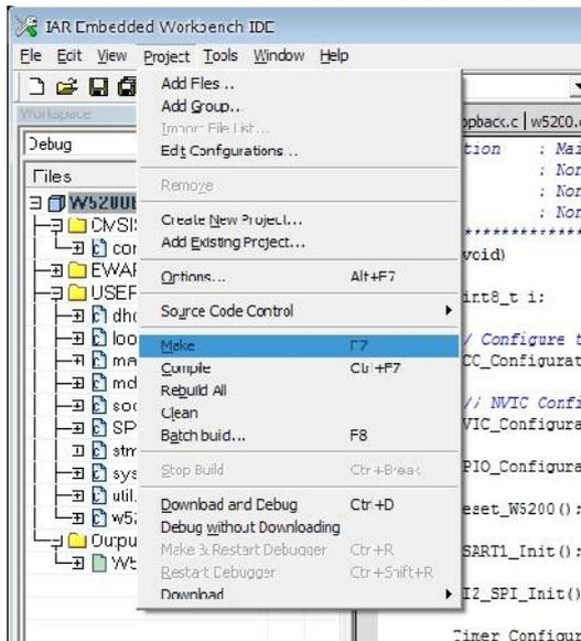
Fig. 4.4 Compile on IAR Embedded Workbench IDE
