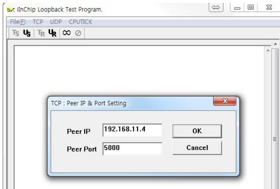
Fig 4.10 AX1 Peer IP & Port Setting
