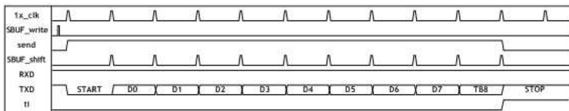
Figure 6.10 Timing Diagram for UART Transmission Mode3
