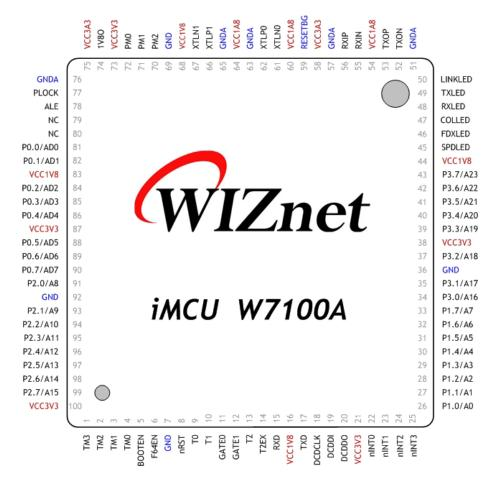
Fig 1. W7100A 100pin LQFP package
