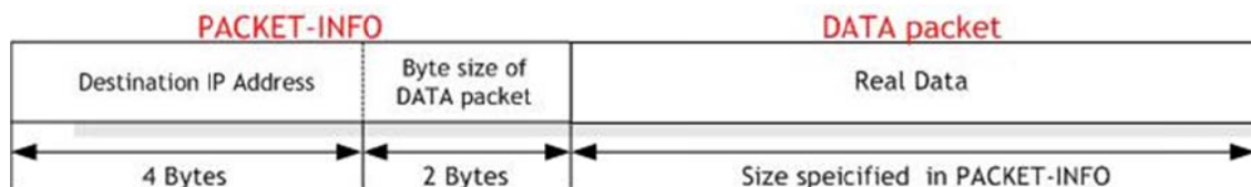
<Fig.2> The received IPRAW data format
