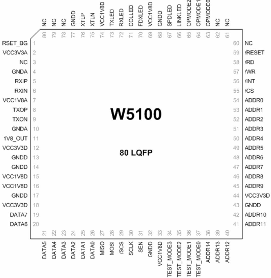
Figure 1. Pinout W5100
