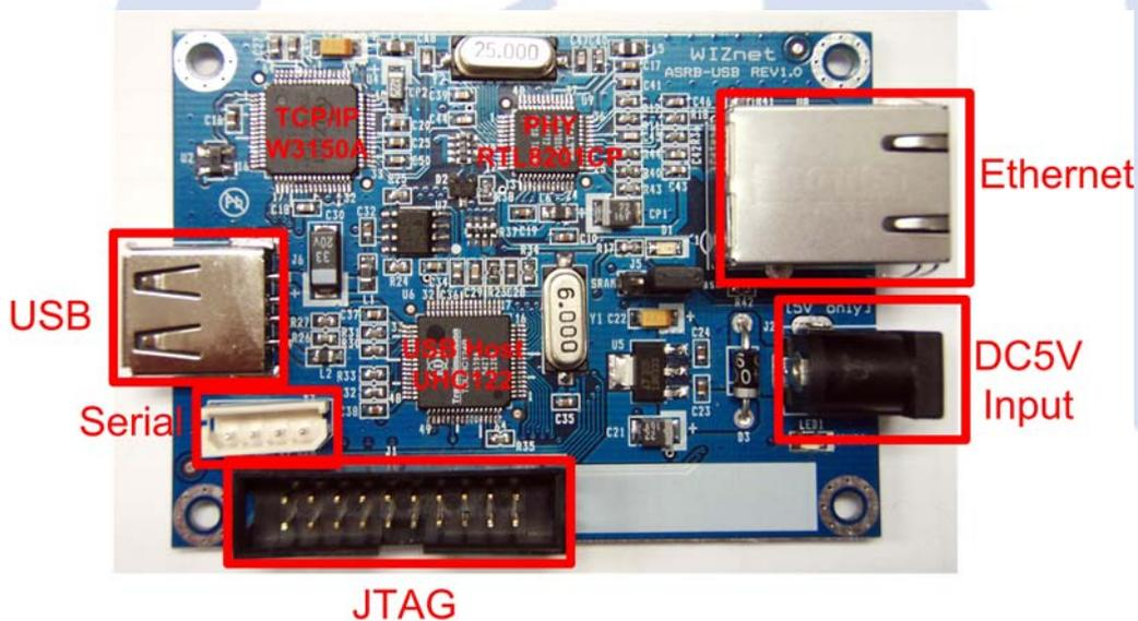
The STR710FZ2 controls the USB host controller and hardwired TCP/IP chip through external memory interface (EMI). The STR710FZ2 is powered by a 3.3V regulator and driven with a single 16MHz clock generator.
