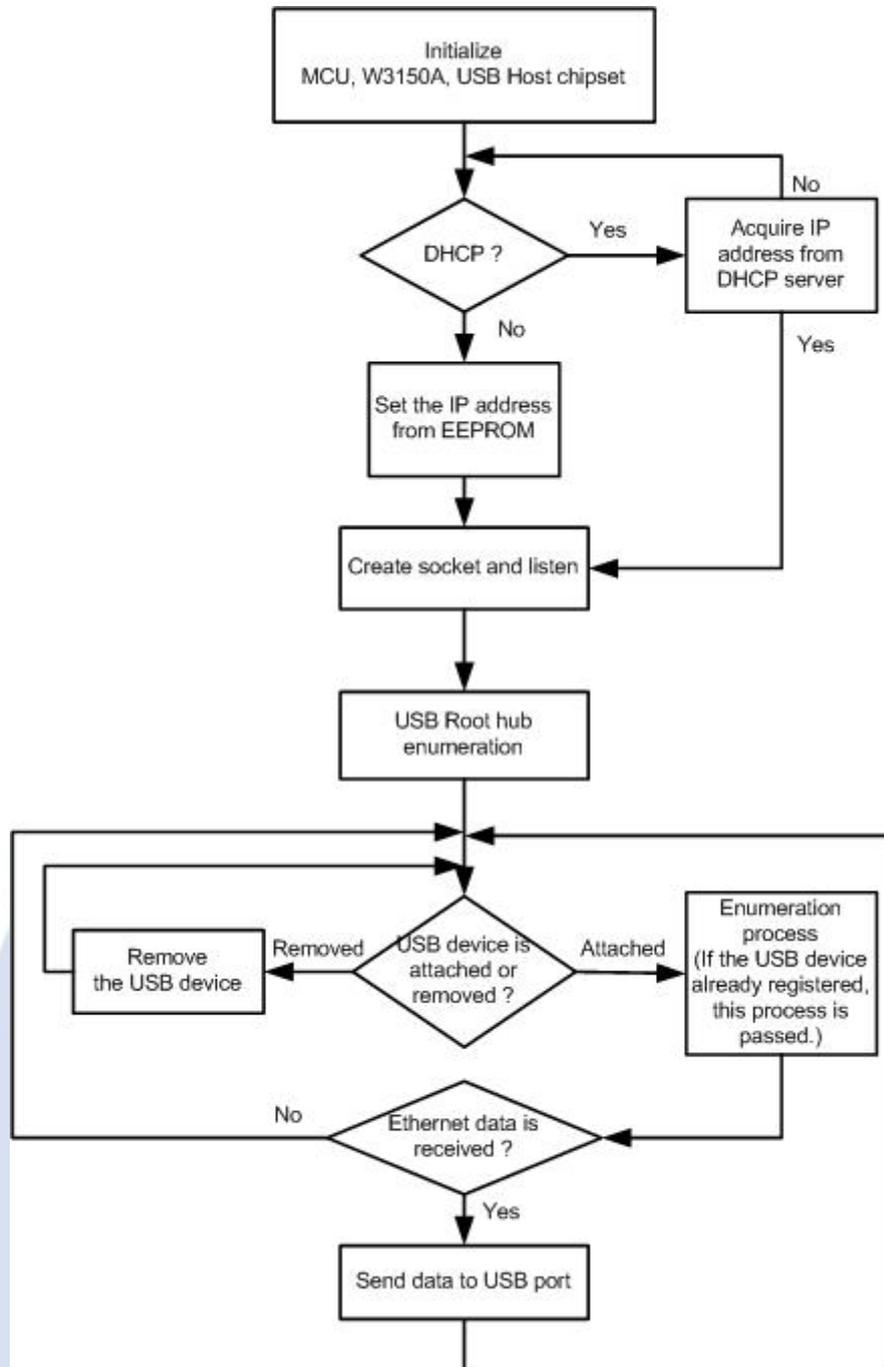
If power is supplied to ASRB-USB board, the basic setting for MCU is processed. Then, W3150A<sup>+</sup> and USB Host chips are initialized. At the DHCP mode, the ASRB-USB will acquire network information from DHCP server. If static IP address is used, the information of the EEPROM will be set. ASRB-USB utilizes sockets for DHCP, communicating with configuration
