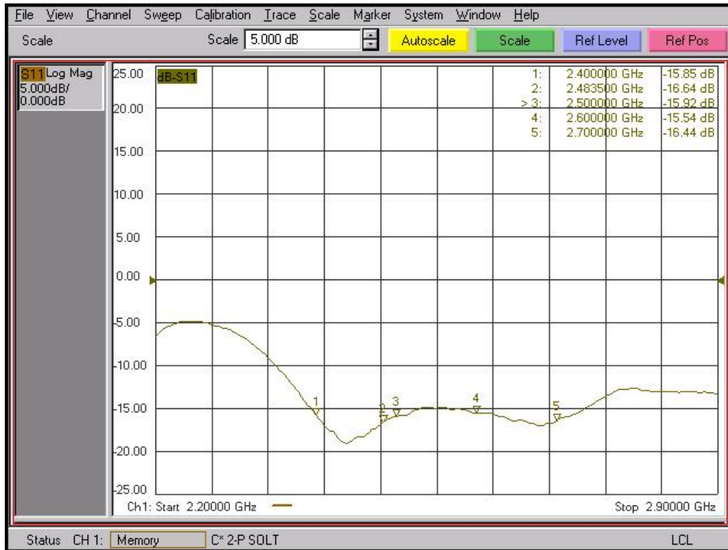
Fig 2. V.S.W.R (Agilent E8358A 300KHz~9GHz PNA Series Network Analyzer)
