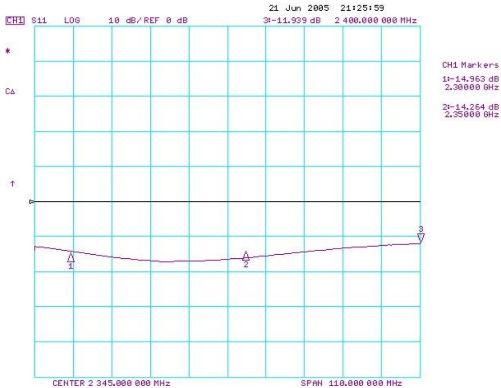
Fig 1. Return Loss (Agilent E8357A 300KHz~6GHz PNA Series Network Analyzer)
