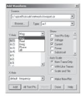
IntuScope enables you to choose the type of waveforms displayed in the pull-down menu under the Y Axis section.
