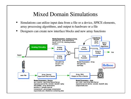
Schematically, SALT objects connect like any other electronic device. The example above contains some basic illustrations. At the top, an input signal is feed into two analog to array blocks which convert the analog information into an array format. One signal is first passed through an analog filter. The array data is summed and then converted back into an analog signal (array to analog block). In this case, the Array Function blocks simply copy data from their input to their output.
