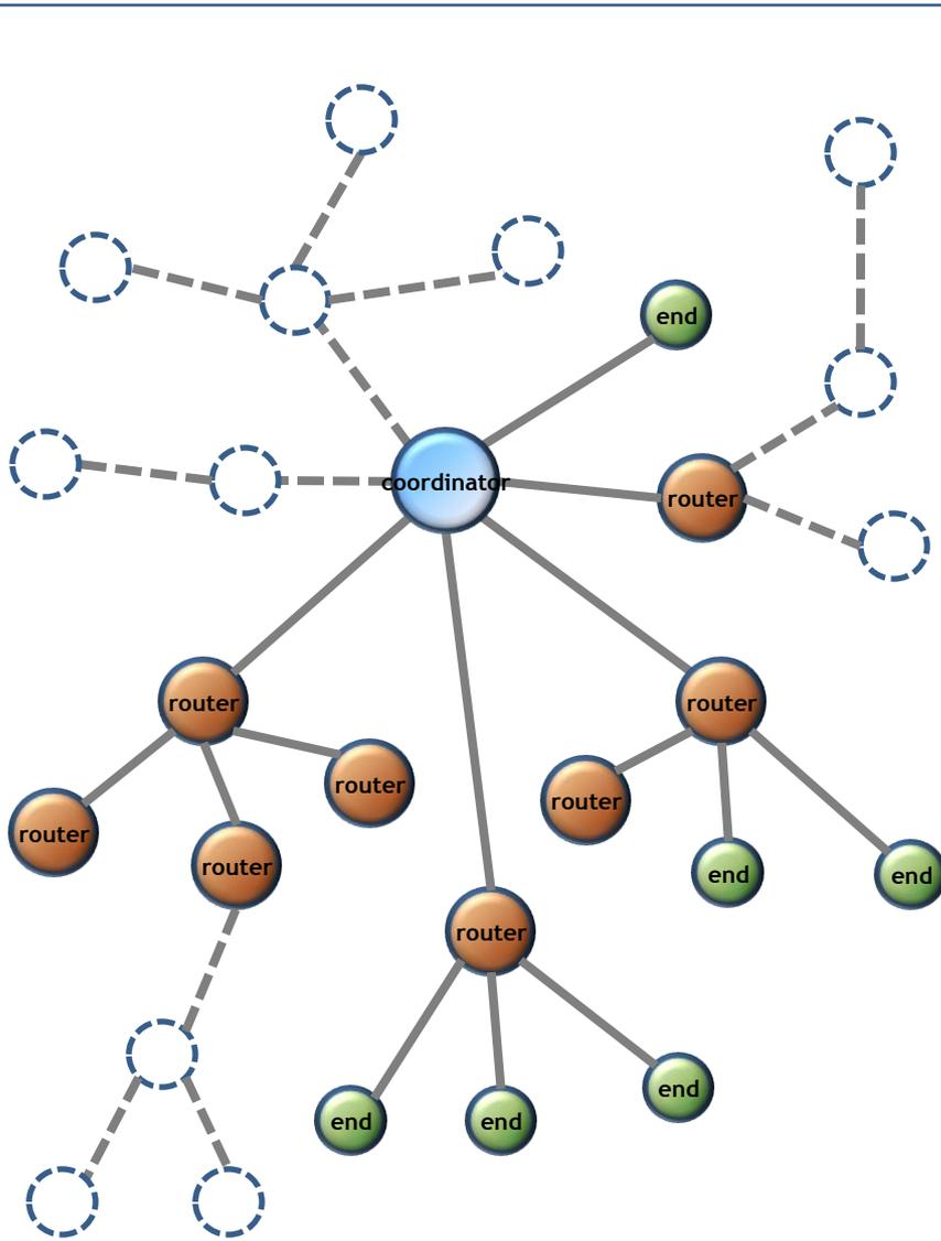
An example of ZigBee Network configuration
