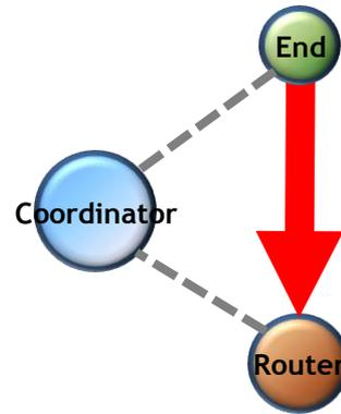
In order to communicate, End Device should be aware of Router's address.
