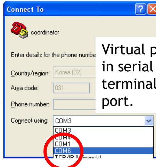
Virtual port connection is possible in serial program like the hyper terminal if there is a virtual serial port.
