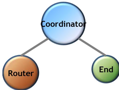
Example 2. Zigbee network construction
