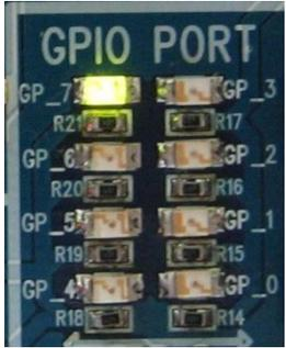
**GP\_7 is ON** when the received data value is GPT00F7.
