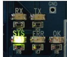
STS LED blinks and ERR/OK LEDs are OFF in the Operation Mode.
