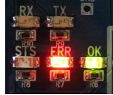
STS LED is OFF and ERR/OK LEDs are ON in the AT Command Mode.
