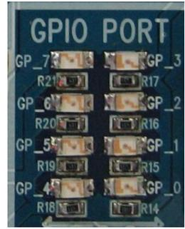
When there is no more incoming GPIO data, the GPIO LEDs will be OFF after a short while.
