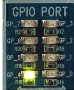
**GP\_4 is ON** when the received data value is GPT00FE.
