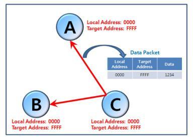
Device A recognizes the data packet as its own data and accepts it since the Target Address of the data packet is FFFF. Device A does not transmit ACK.
