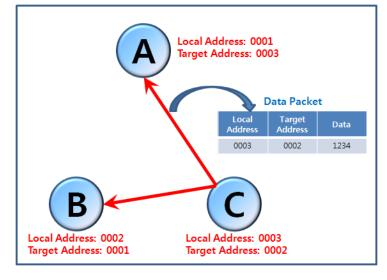
Device A does not recognize the data packet as its own data since the Target Address of the data packet is 0002 and ignores it.
