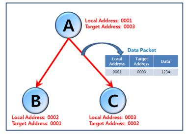
Device B does not recognize the data packet as its own data since the Target Address of the data packet is 0003 and ignores it.
