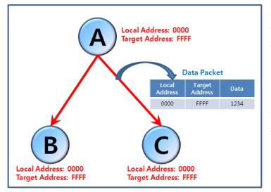
Device B recognizes the data packet as its own data and accepts it since the Target Address of the data packet is FFFF. Device B does not transmit ACK.
