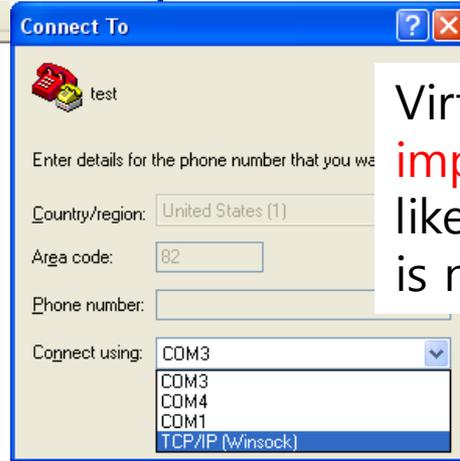
Virtual port connection is impossible in serial program like the hyper terminal if there is no a virtual serial port.
