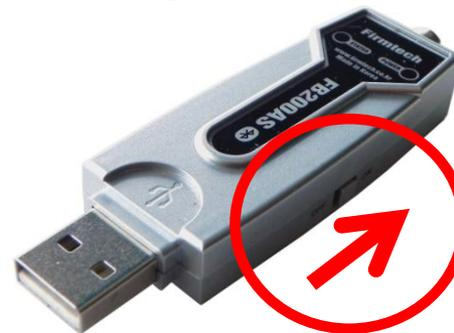
There is "virtual serial port in "port agenda" if a power-supply of FB200AS is ON.
